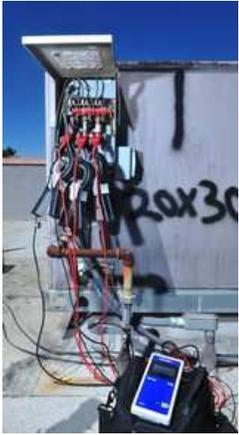
Photo by Joseph A. Garcia / Star staff Testing of an air conditioning unit with the AircoSaver device, which will show its voltage and current, begins. Several air conditioning units were tested before and after they were retrofitted with the AircoSaver device.
